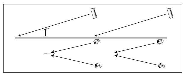
Figure 16 - Measurement Microphone Placement for Auto EQ of Aux Speakers 3A and 4B
